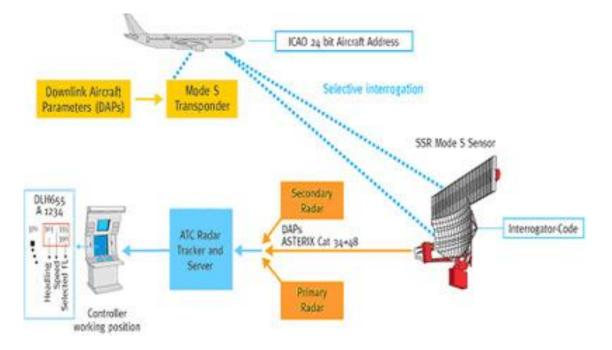
In parts of Europe, there have been mandates issued requiring all aircraft that fly into designated airspace to be equipped with a Mode S transponder capable of supplying aircraft derived data.
